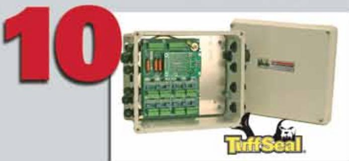
**Rice Lake TuffSeal™:** Fiberglass Reinforced Polyester (FRP) FRP Junction Box enclosure features a "Gore"™ PreVent membrane that equalizes the inside and outside pressure. Water is repelled but a special hydrophobic (water-fearing) membrane continuously allows condensation to escape.
