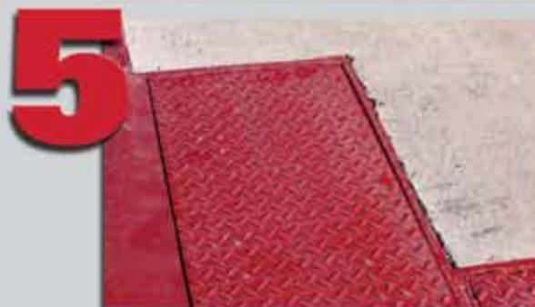
**Stronger Weighbridges:** Rice Lake truck scales typically have up to 30% more structural steel content than competitive models. The SURVIVOR<sup>®</sup> OTR 11' wide model uses (2) 12" wide flange, 14 lbs per foot main beams, (7) 6" wide flange, 9 lbs per foot support beams per module, 3/16" lower plate and Nelson studs. Less bridge deflection means longer scale life.
