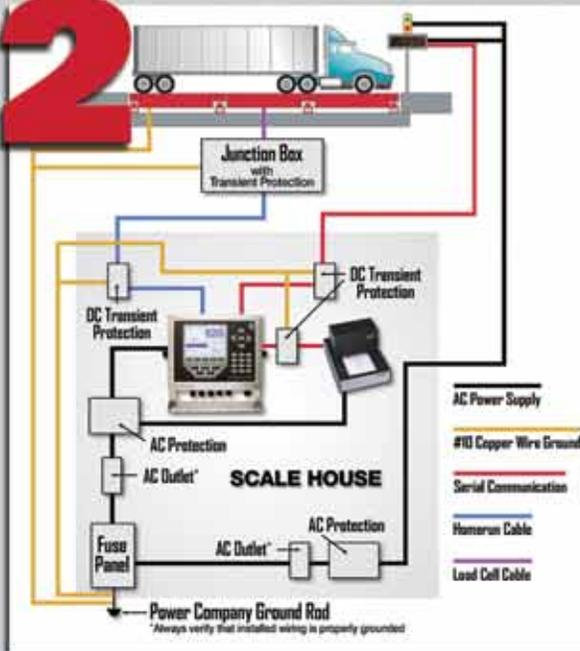
**Lightning Protection:** Every SURVIVOR® Truck scale comes complete with a Surge Voltage Protection System that includes a UPS 2000 Sola Duplex Transformer. The junction box is provided with individual UJB-3T6 DC transient circuitry protection. The entire system is grounded to a single-point grounding system connected to the power ground. Our scales come with a five-year warranty on the load cells and junction box, and either a five- or ten-year warranty on the weighbridge.
