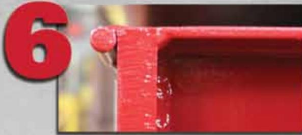
**Rock Guards:** are welded to perimeter of scale for pit installations, and ends of scale for top of ground installations. Small rocks that can wedge between the head wall or side walls causing scale errors are eliminated.
