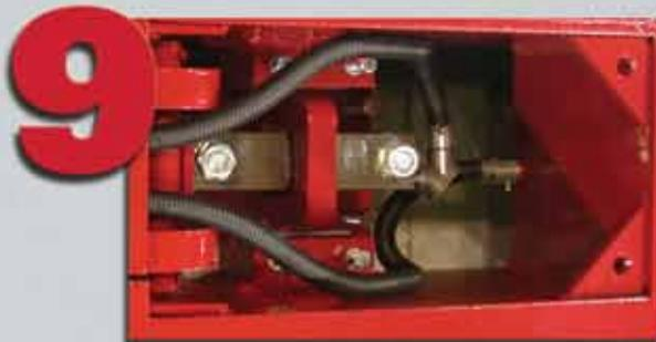
**Rugged 75,000 lb Capacity Load Cells:**
