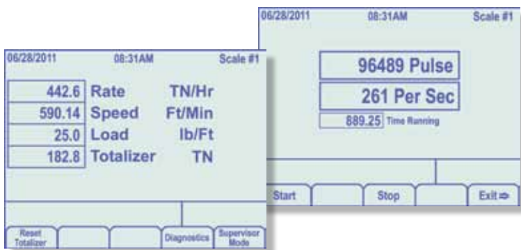
Easy-to-read display shows rate, speed, real-time load, and total material weighed across the belt since last reset. Configuration is intuitive and fast.
