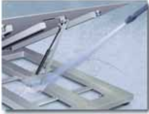
The rugged design incorporates 304 stainless steel construction and four welded-seal load cells with PTFE cable designed for high temperatures and washdown areas.
